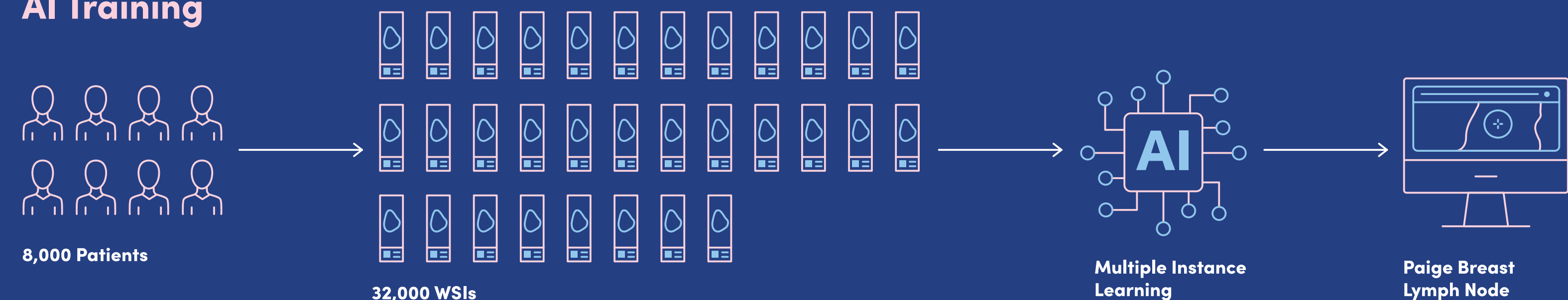
Fig 1. AI algorithm training. More than 32,000 breast sentinel lymph node WSIs from more than 8,000 patients were used to train Paige Breast Lymph Node, a deep learning algorithm trained using multiple instance learning, a weakly supervised approach that couples the WSI image with the corresponding pathology report and does not require manual annotations.
